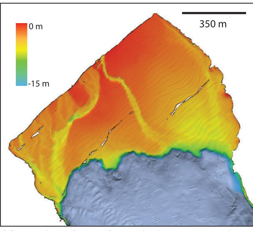
delta top channel network: note the direct connection between bedforms and western channel mouth
