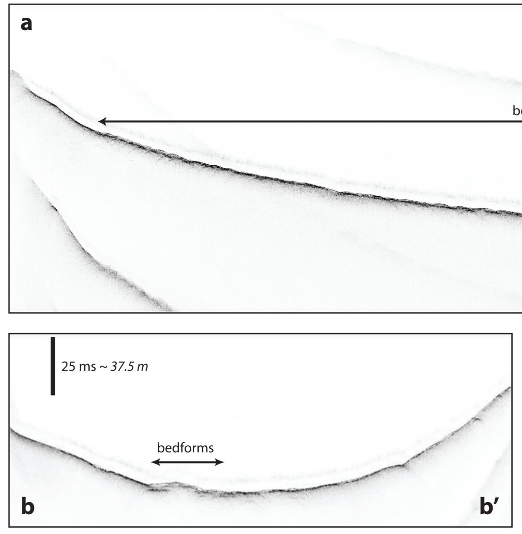
**2. The bedforms:** due to the poor acoustic penetration, the internal structure of the bedforms is not well imaged. The data do indicate, however, that the bedforms are associated with a bathymetric high (see line b-b'). Whether this high is due to aggradation of the bedforms, or thickening associated with mass failure is unclear.
