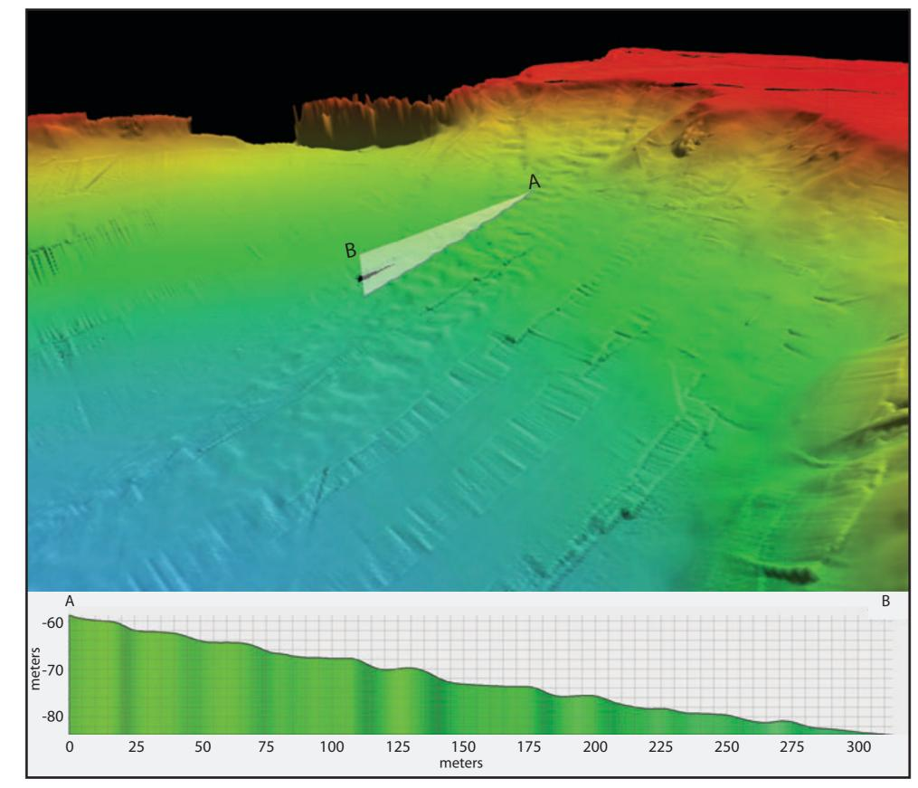
perspective view (looking west) of bedforms: note the average wavelength ~25m and average amplitude ~1m in this area
