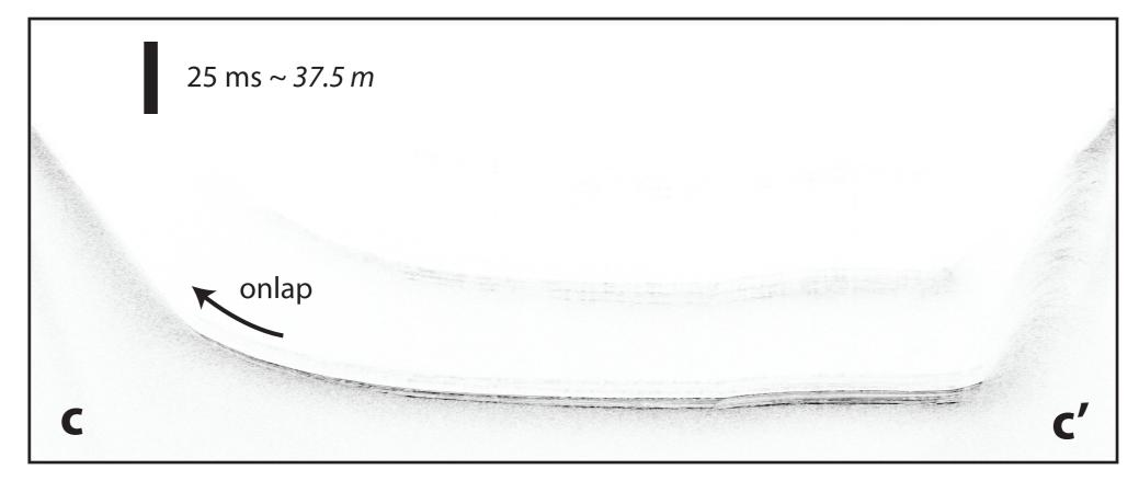
3. Lateral depositional trends: The chirp data indicate that distal flatlying sediments thin and onlap onto the steep sides of the lake, in a manner consistent with deposition by relatively thick (10s of m) turbidity currents (see line c-c').
