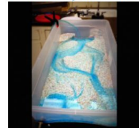
DIY Recirculating Stream Table
