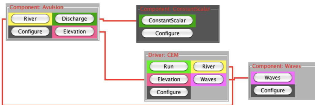
Wiring Diagram for coupled CEM-Avulsion-River simulations
