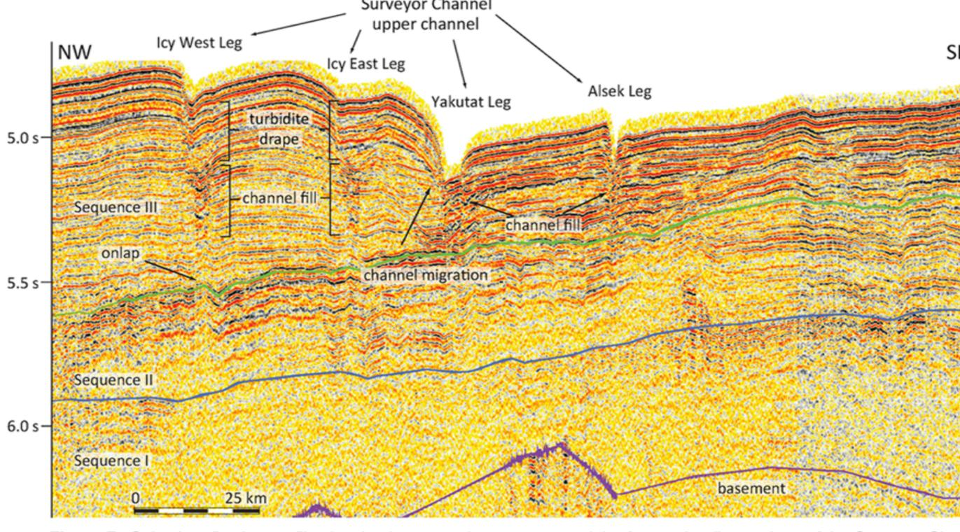
Figure 7. Seismic reflection profile showing interpreted sequences and the four main tributary legs of the Surveyor Channel. See Fig. 3 for line location. Vertical axis in two-way travel time. Vertical exaggeration ~50:1 assuming 2000 m/s sediment acoustic velocity. (USGS Survey F789)
