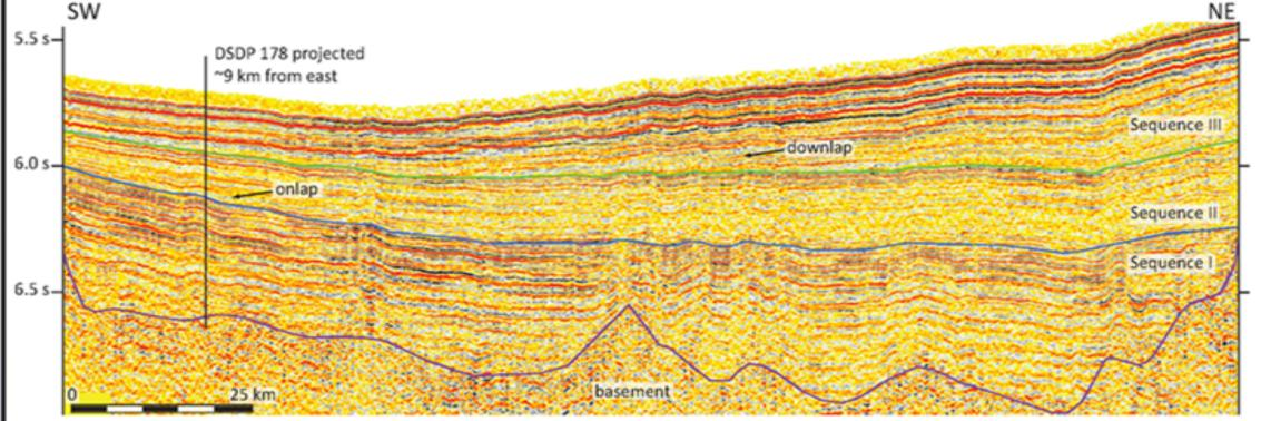
Figure 4. Seismic reflection profile showing interpreted sequences and approx. correlation to Deep Sea Drilling Project (DSDP) Site 178. See Fig. 3 for line location. Vertical axis in two-way travel time. Vertical exaggeration ~35:1 assuming 2000 m/s sediment acoustic velocity. (USGS Survey
