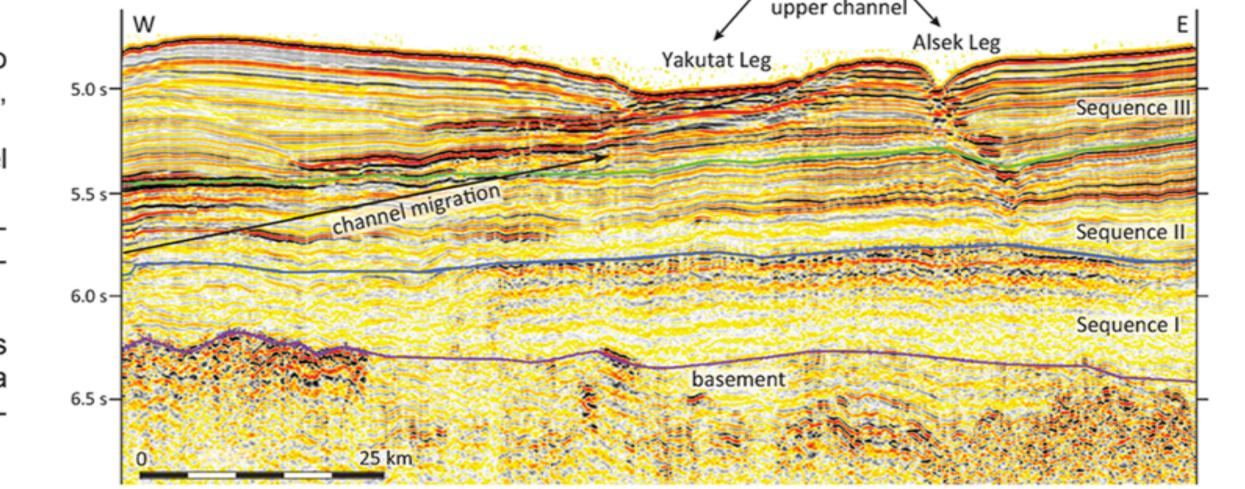
Figure 5. Seismic reflection profile showing interpreted sequences and migration of the Yakutat Leg of the Surveyor Channel. See Fig. 3 for line location. Vertical axis in two-way travel time. Vertical exaggeration ~20:1 assuming a 2000 m/s sediment acoustic velocity. (USGS Survey L378)
