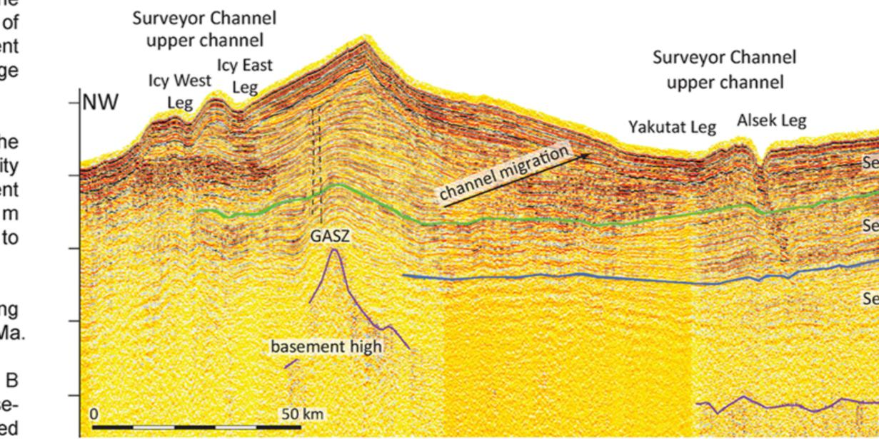
Figure 9. Seismic reflection profile showing interpreted sequences and four main tributary legs of the Surveyor Channel. Also evident is the basement high and sediment wedge that influenced migration of the Yakutat Leg. GASZ-Gulf of Alaska Shear Zone (e.g., Gulick et al., 2007). See Fig. 3 for line location. Vertical axis in two-way travel time. Vertical exaggeration ~35:1 assuming 2000 m/s sediment acoustic velocity. (USGS Survey F689)
