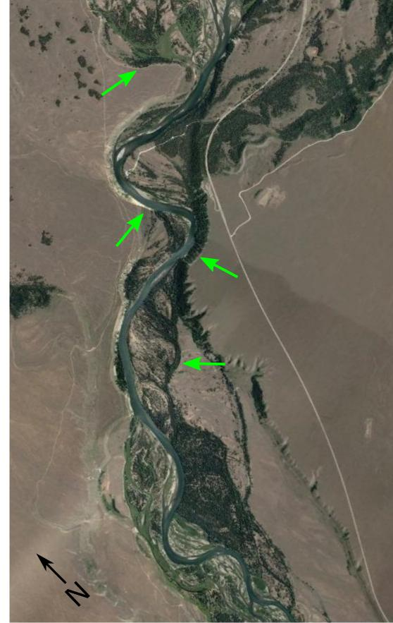
Example of possible current and past DSE of terraces on the Snake River, Grand Teton NP. Terraces erode on downstream sections of bends and meanders migrate downstream.
