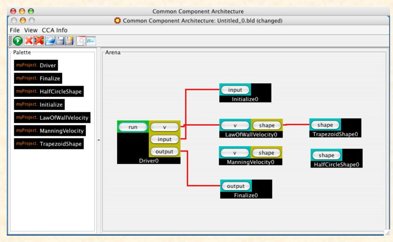
A "wiring diagram" for a simple CCA project. The CCA framework called **Ccaffeine** provides a "visual programming" GUI for linking components to create working applications.
