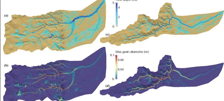
Figure 5: Simulation results of the 2013 Front Range flood on Boulder Creek (left) and Lefthand Creek (right) for September 12 at 4:00 PM. (Top) Flow depth, (Bottom) Maximum transportable grain size, obtained from the shear stress that the flow could impart on the bed given the flow depth and momentum produced by the hydrodynamic model.
