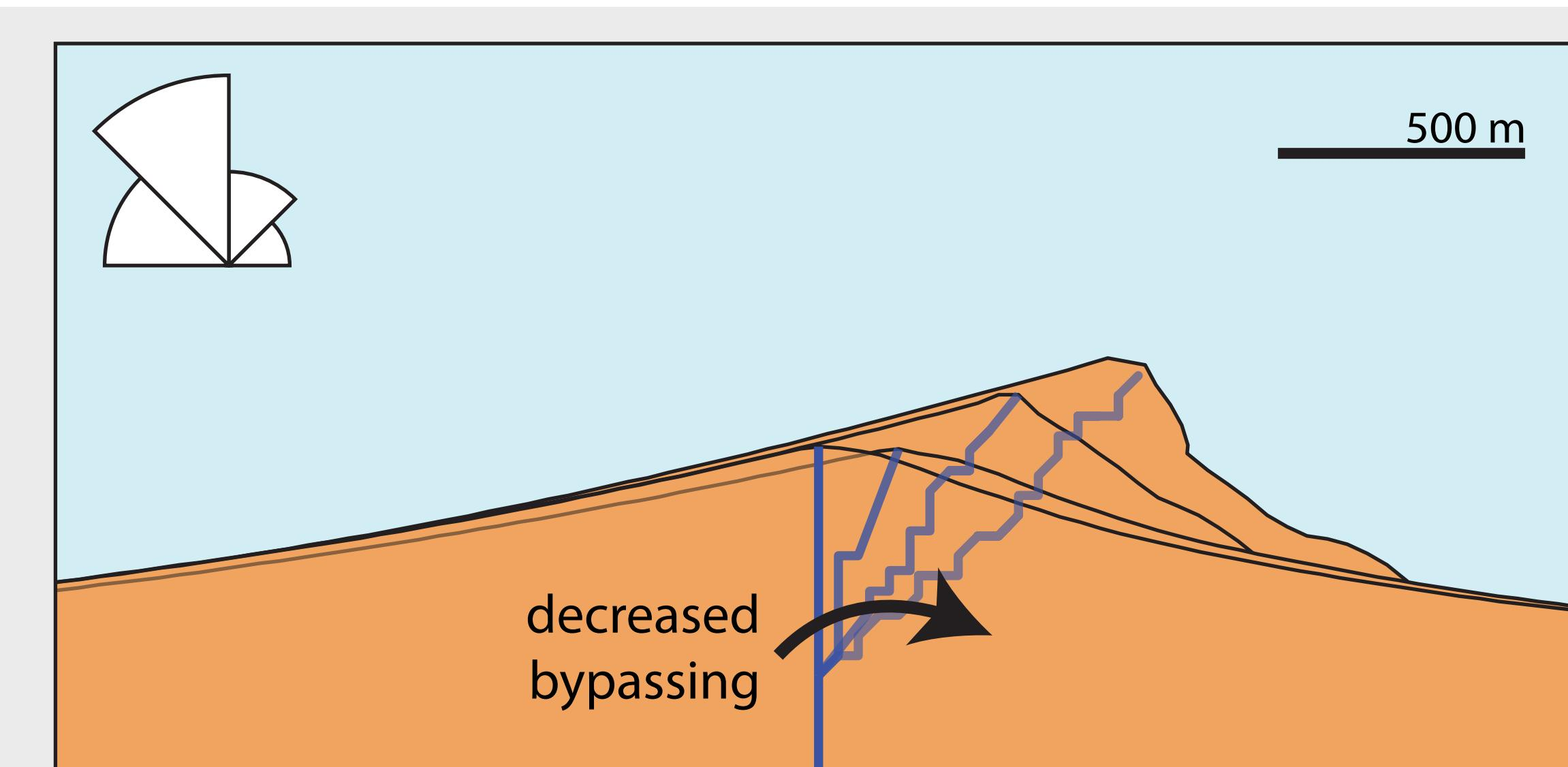
Channels only deflect away from waves if the river mouth obstructs alongshore transport. The fraction of sediment that is allowed to bypass influences channel orientation.
