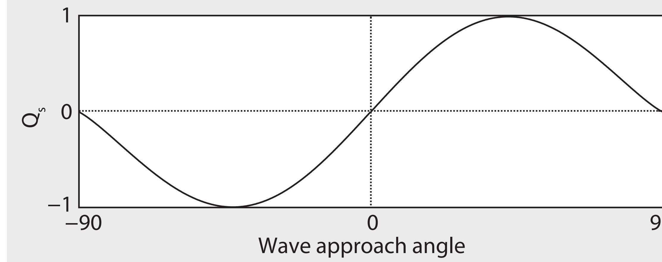
Littoral transport is a function of wave approach angle, setting up a feedback with the changing shoreline orientation of a delta [Ashton & Murray, JGR, 2006]
