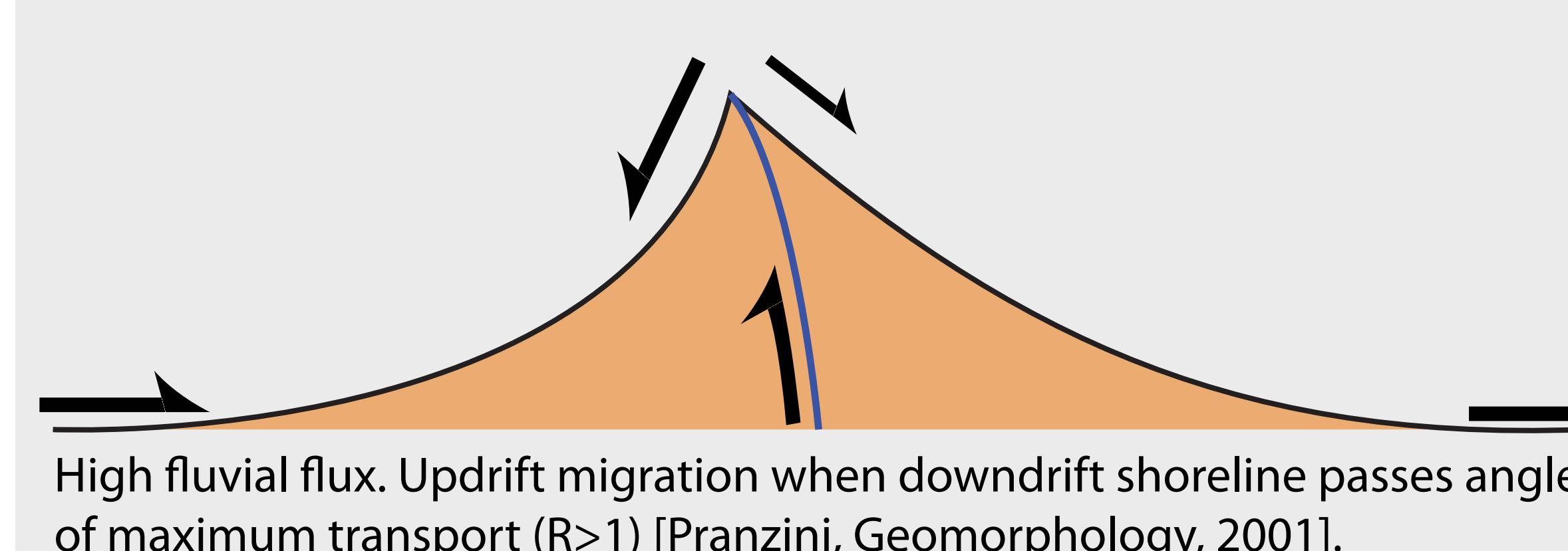
High fluvial flux. Updrift migration when downdrift shoreline passes angle of maximum transport ( $R > 1$ ) [Pranzini, Geomorphology, 2001].
