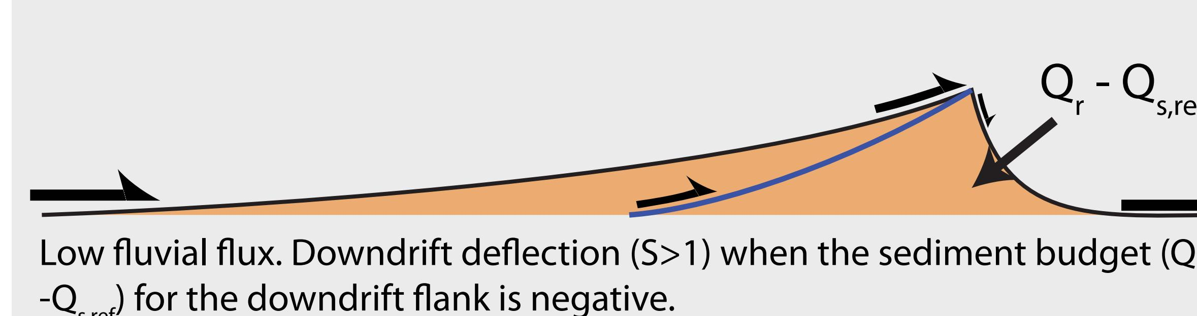
Low fluvial flux. Downdrift deflection ( $S > 1$ ) when the sediment budget ( $Q_r - Q_{s,ref}$ ) for the downdrift flank is negative.
