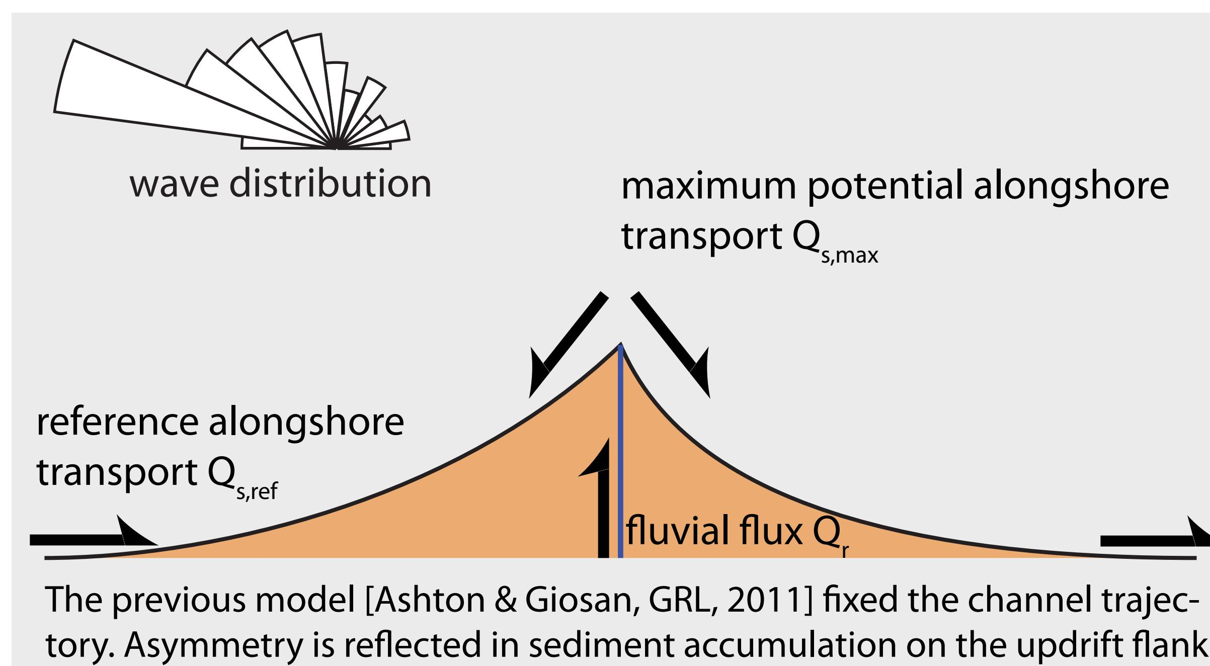
The previous model [Ashton & Giosan, GRL, 2011] fixed the channel trajectory. Asymmetry is reflected in sediment accumulation on the updrift flank.
