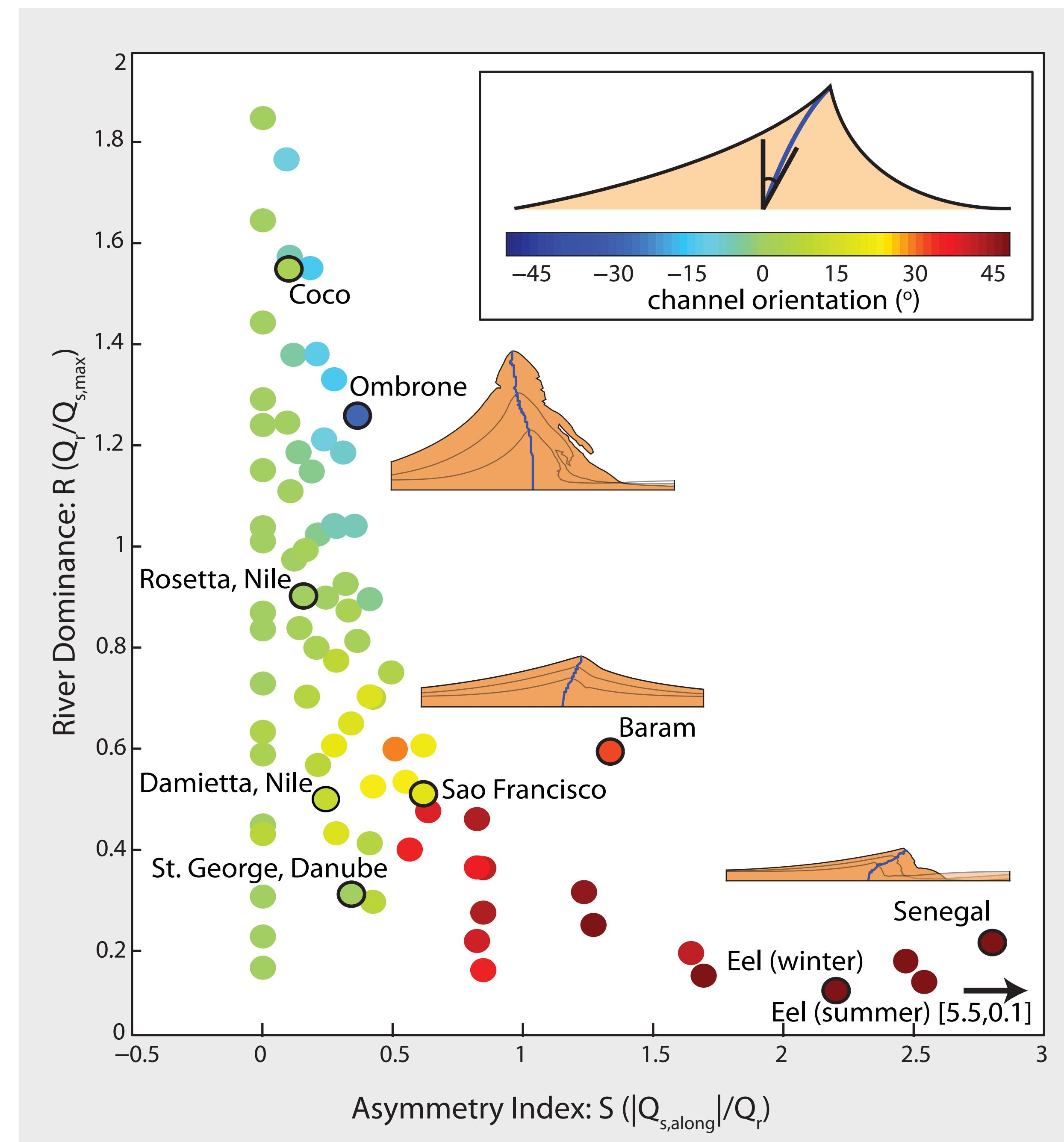
Two new indices explain the spread of channel angles seen in modeled and natural examples.
