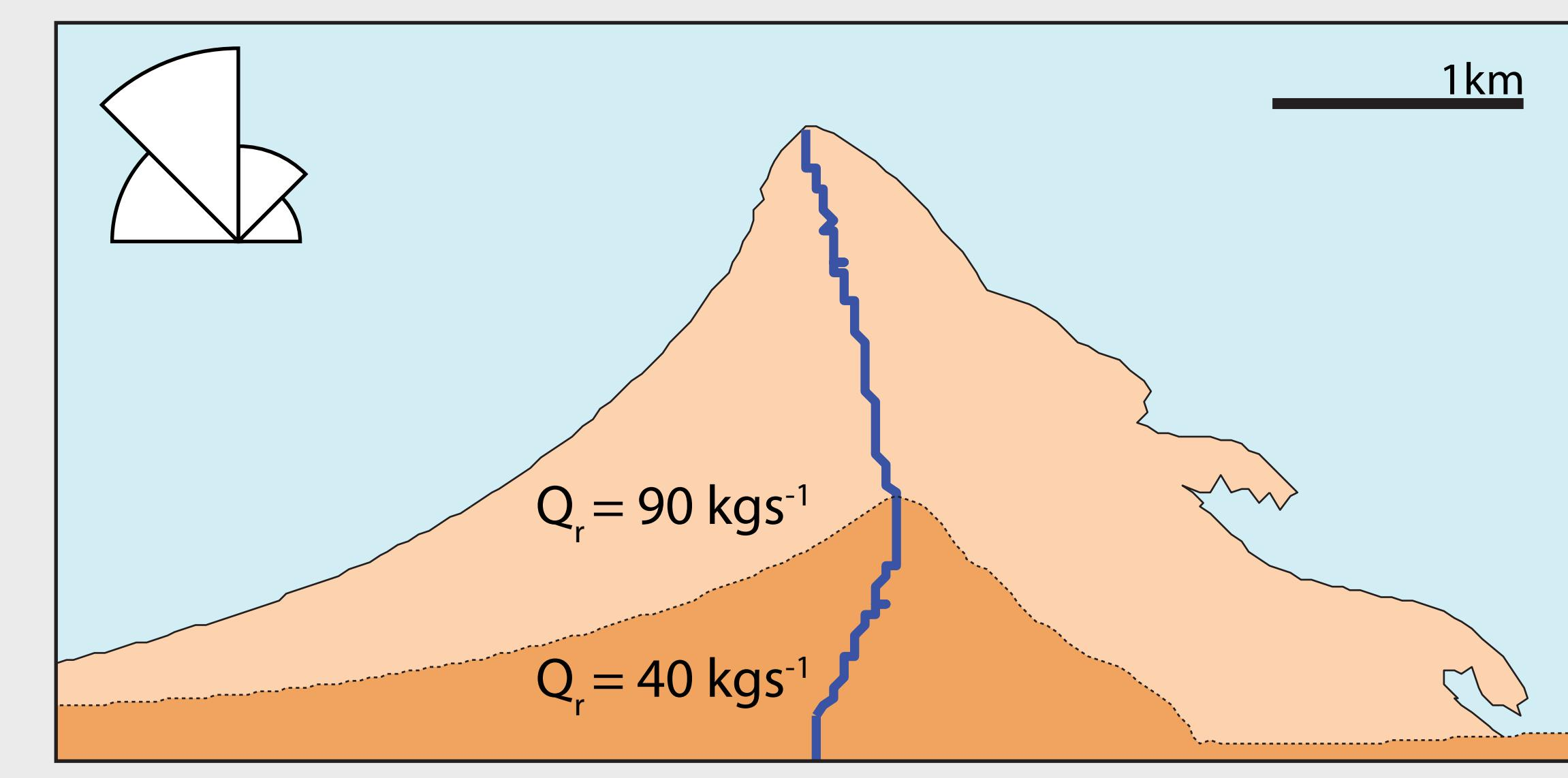
Channels can change orientation as a response to a change in fluvial sediment supply [see Pranzini, Geomorphology 2001].
