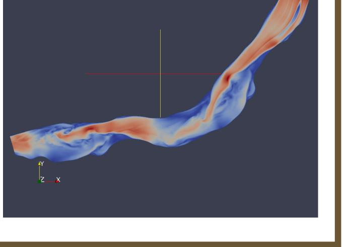
Latest results of the CFD modeling. Eminence Break and Willie Taylor eddy fan complexes. Upstream velocity boundary condition imposed to generate fully developed turbulence at the inlet.
