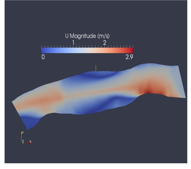
Flow field solved using Detached eddy simulation (DES) approach. Time: 1000 secs
