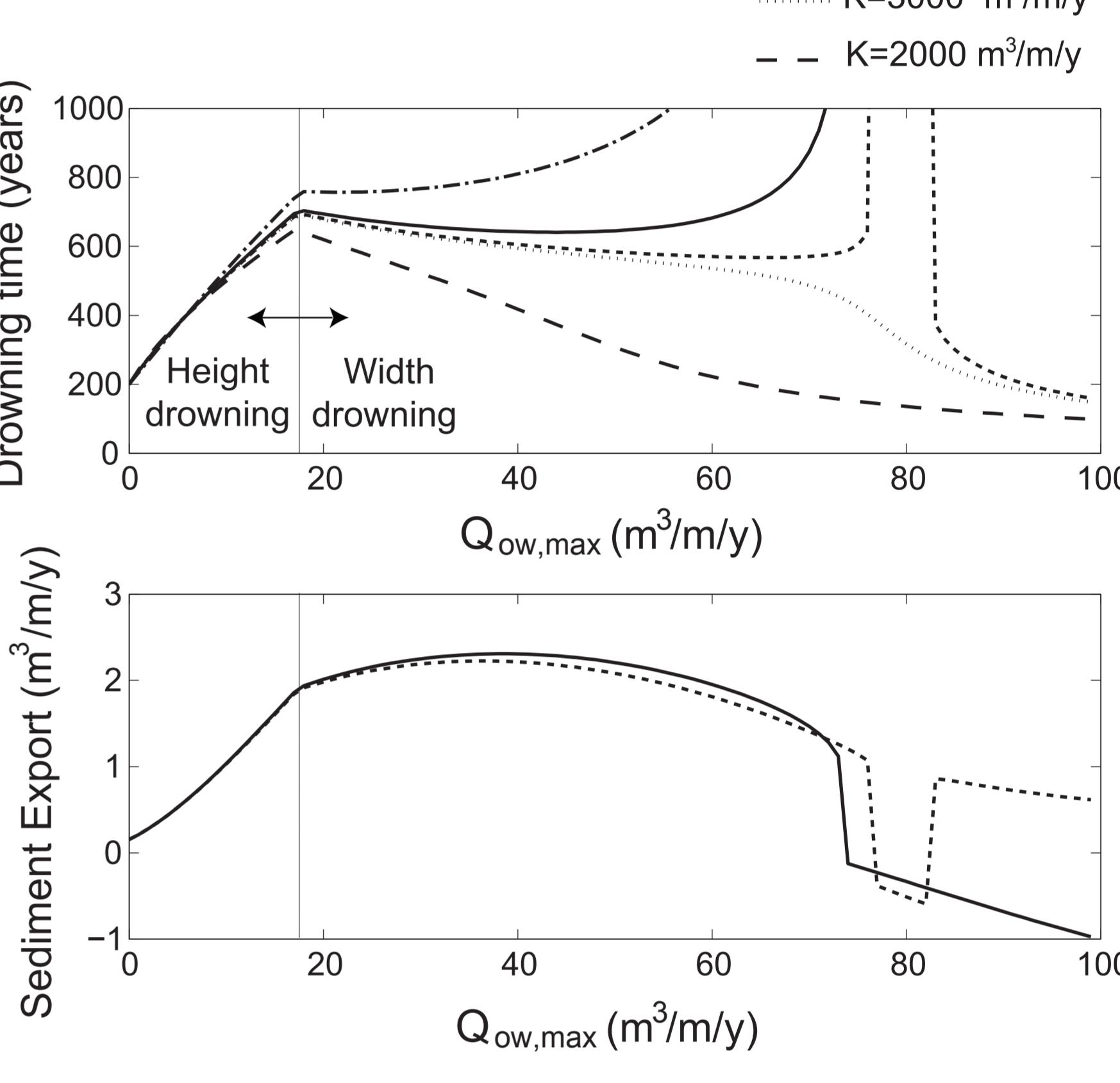
**Height drowning** is numerically identified when the barrier height is completely submerged (i.e.,  $H < 0$ ).
