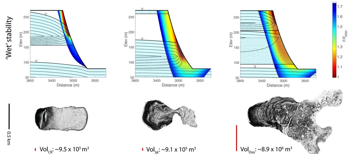
Each terrace shows a unique signature of stability dictated by its stratigraphic configuration. In the Cedar and NFSR cases, the stratigraphic pattern becomes uniformly less stable with groundwater flow. In the Skagit case, this pattern is altered by high pore-fluid pressures at its base.
