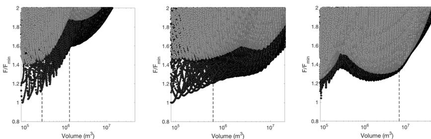
Left: Plots showing volume and factor of safety for each modeled potential failure plane within Scoops3D. Grey dots are 'Dry' runs and black dots are 'Wet' runs.
