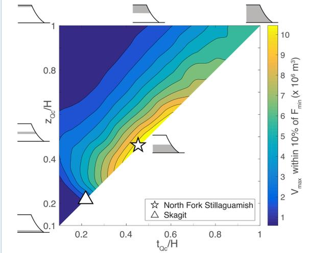
We model landslide volumes by varying the position and thickness of a weak clay unit within an outwash terrace, and find that the largest landslides occur in terraces with 40-60% Qc along their bases like the North Fork Stillaguamish configuration.
