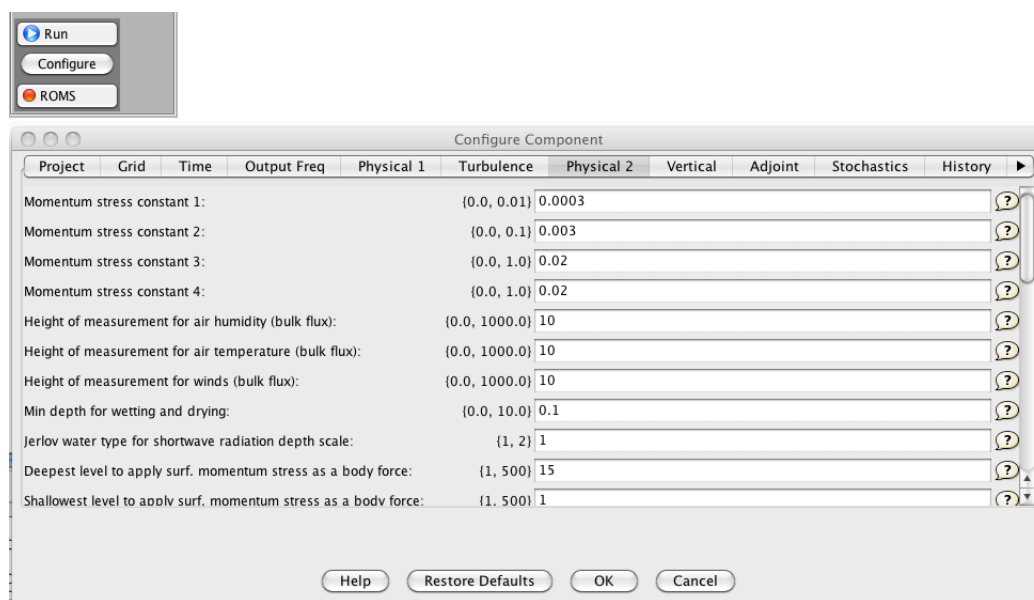
Figure 3.7. ROMS-the Regional Ocean Modeling System can be run stand-alone in CMT. Users click on the 'configure' tab and set simulation parameters. The 'help' button on the bottom-left leads to advanced documentation on model setup and parameters. Given ROMS vibrant user-base and documentation on its wiki website, the 'help' her leads to the MyROMS community user page.
