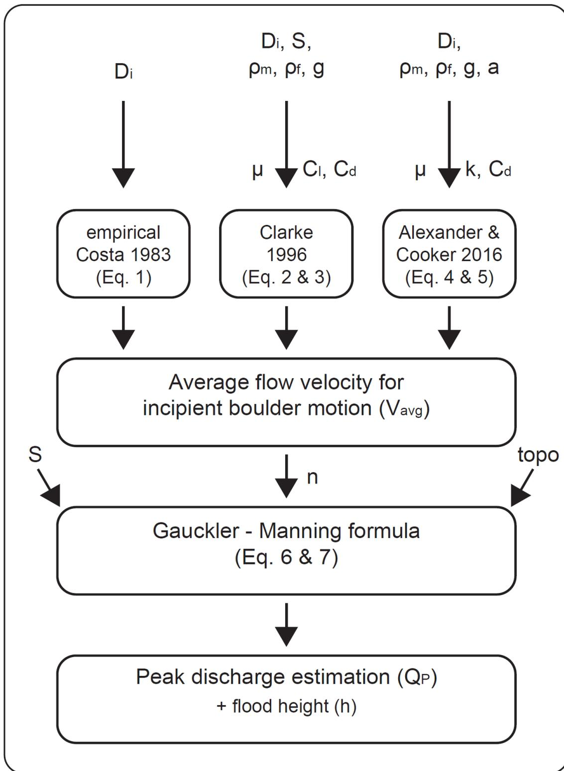
Figure 1: Flow-chart showing steps of computation for *allochthonous\_boulders\_for\_paleohydrology.m* and *compare\_VQh.m* codes. General input parameters on very top together with input coefficients below next to arrows. Compare with equations above. Topographic input (topo, S) is not added until Gauckler-Manning formula is applied.
