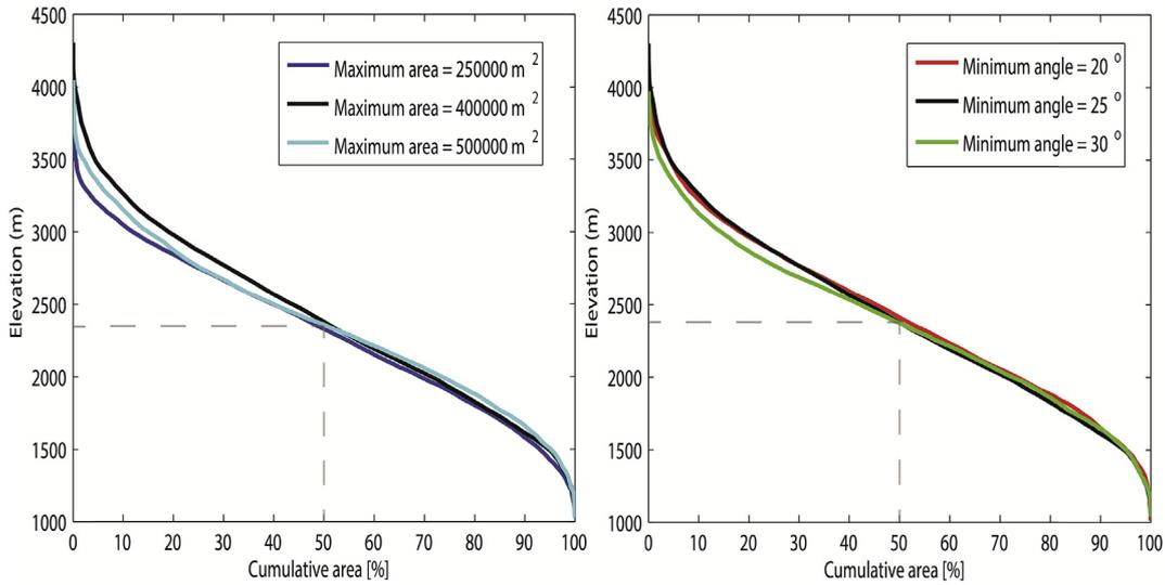
**Fig. 11.** Hypsometric curves of the cases with different minimum interior angle and maximum area. Left: hypsometric curves with the same minimum angle but different maximum area. Right: hypsometric curves with the same maximum area but different minimum angle. Although the plots show a difference at the top of the hypsometric curve, the value and pattern are almost invariant with different mesh structure.
