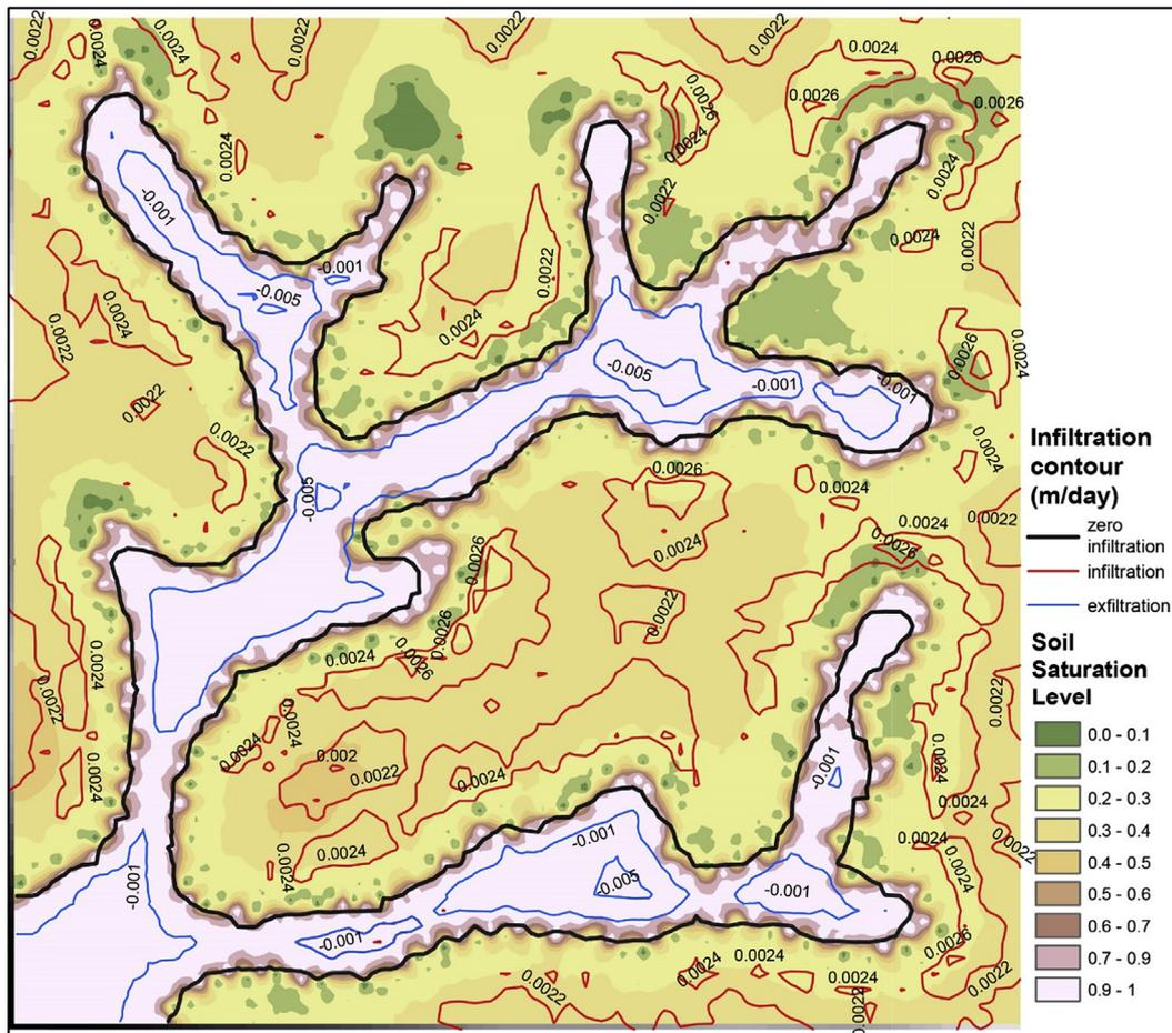
Fig. 8. Spatial distribution of infiltration and exfiltration (the rate in unit of meter per day).
