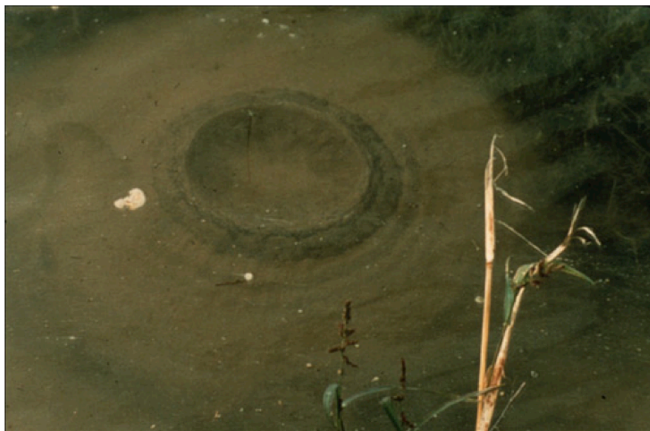
Figure 12 CSDMS YouTube movie to explain the concept of a sand boil near a river levee as a result of flood discharge and pressure gradients between the river channel and the surrounding floodplain. Posted during the May 2011 Mississippi floods.
