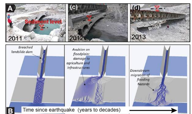
(A) an example of the dramatic impacts of the post-seismic river aggregation on infrastructure following the 2008 Mw 7.9 Wenchuan earthquake, China (Zhang et al. 2016). (B) EROS model demonstrating the potential for modelling the catchment scale flooding responses to earthquake induced landslides and landslide dams (Davy et al. 2009)
