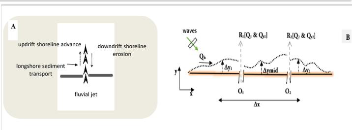
Figure 1: Schematic illustration of waves action against fluvial discharge along the delta coastline
