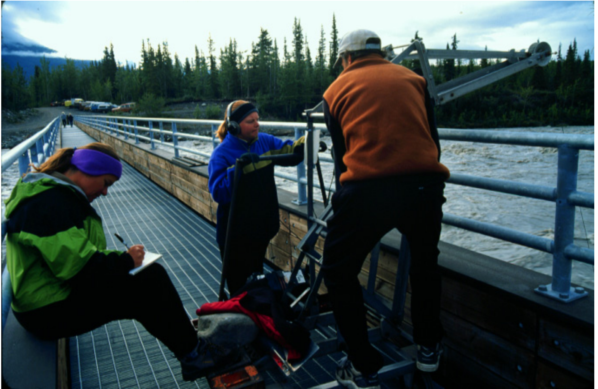
Measuring the Kennicott River discharge
