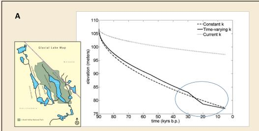
Fig. 1 (A) Curves comparing rates of elevation loss (degradation) using long-term average constant K and time varying K at a single location, Mono Basin, CA (Madoff and Putkonen, 2016) and map (Jol, 2007) showing connectivity of glacial lake basins that proxy climate record is taken from (Lowenstein, 1999).
