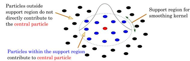
SPH is able to handle the fluid accelerations very well, which allows for robust solutions of the inertial N-S term and realistic simulation of fluid-structure interaction. Simulation of millions of particles with DualSPHysics (Crespo et al., 2015) enables investigation of the forces and kinematics associated with flow past heterogeneous boundaries in three dimensions.
