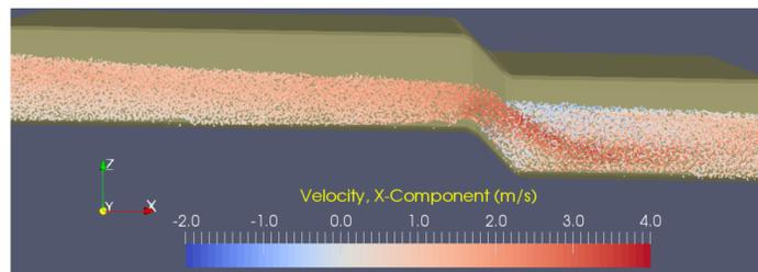
Figure 6 shows the velocity structure of the flow field across the knickpoint, which was calculated using 104,154 SPH particles. There is a strong return flow (up to 2 m/s) at the knickpoint.
