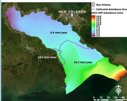
Figure 2: Subsidence spatial distribution. The background raster represents the 2023 CMP combined shallow and deep subsidence rates. The numbers represent calibrated subsidence values based on the 2017 CMP (Khalifa et al., 2024). The dashed lines represent the division between the different calibrated subsidence zones.
