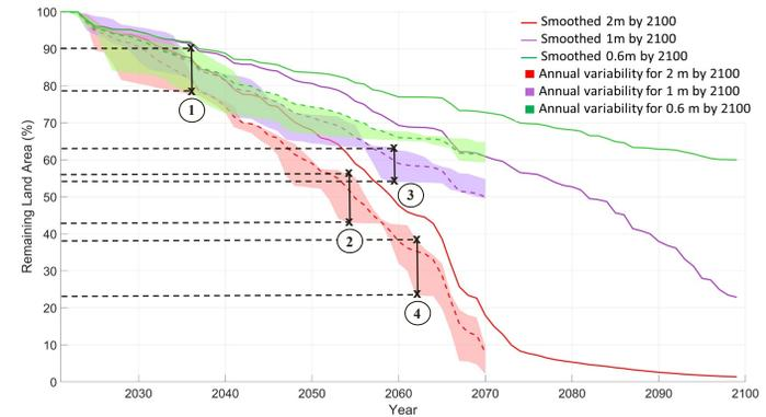
Figure 5: Remaining land percentage [with marsh edge erosion based on Reed et al., (2020) as the dashed colored lines]. Modeled land areas due to annual variabilities are plotted around scenarios with marsh edge erosion as shaded polygons.
