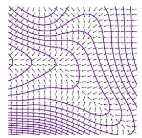
Fig. 18.6: Continuous-angle flow vectors in the vicinity of a channel junction or fork, extracted using the Mass Flux method. (⑦ Rivix, LLC, used with permission)
