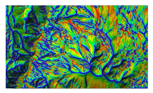
Fig. 18.5: A relief-shaded image of a TCA grid for Mt. Sopris, Colorado, that was created using the Mass Flux method. Areas with a large TCA are shown in red while areas with a small TCA value (e.g. ridgelines) are shown in blue and purple. Complex flow paths are clearly visible and results are superior to both the D8 and D-infinity methods. (© Rivix, LLC, used with permission)
