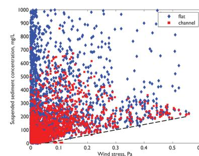
Wind stress is an effective indicator for minimum (i.e., background) SSC in both secondary channels and flats. Background SSC increases linearly with wind stress (left figure), indicating that wind, and by proxy, wind-generated waves, keeps sediment in suspension that otherwise would have settled out of the water column.
