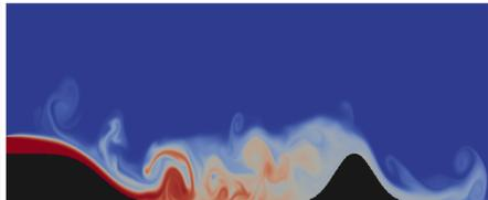
Left: Particle concentration contour for a turbidity current flowing into a mini-basin and interacting with a hump. Transient deposit profiles, interaction of the current with the hump, vortical structures and etc can be studied via TURBINS.
