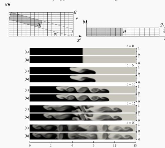
Comparison of the gravity current concentration fields (white corresponds to  $c = 0$  and black to  $c = 1$ ) in a sloping channel with  $\theta = 15^\circ$  and  $Re_H = 750$ , obtained via two different numerical approaches. a): present immersed boundary approach, b): coordinates aligned with container walls.
