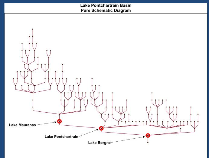
The diagram provides a simplified depiction of the topology of the Lake Pontchartrain Basin. Up and downstream traces can be executed and transferred to the map.
