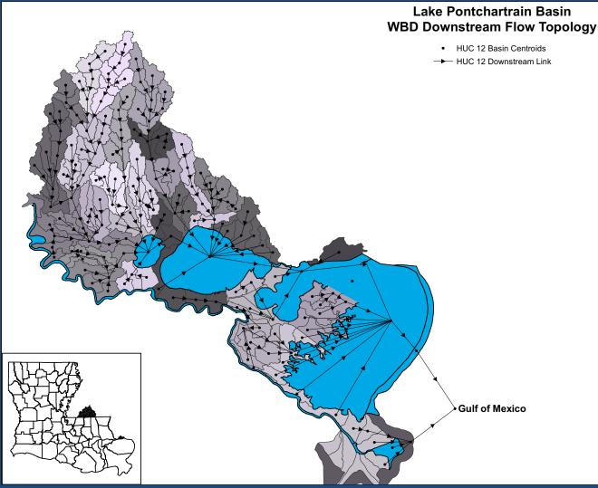
A schematic visualization of the basin drainage pattern. This clearly depicts the drainage network in geographic space.
