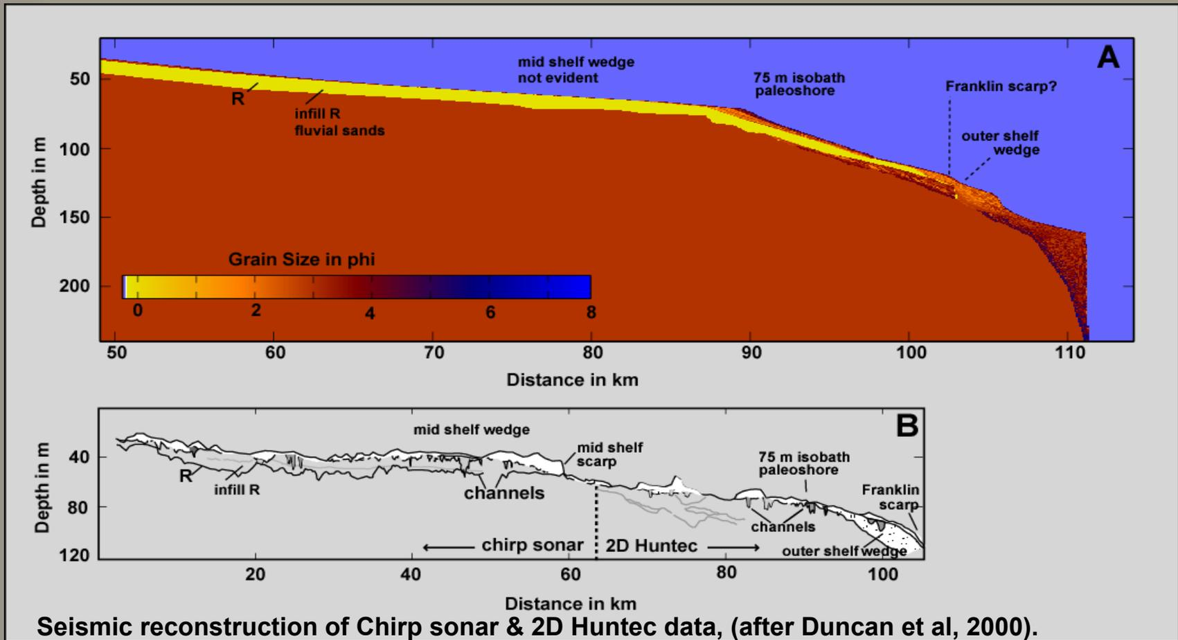
Simulation shows a sea-level-rise controlled retrograding system. Late Pleistocene deposition is high and leaves an extensive deltaic wedge close to the shelf slope at 110 km. Intense storm reworking moves the depocenter of the delta to ~160 m water depth.
