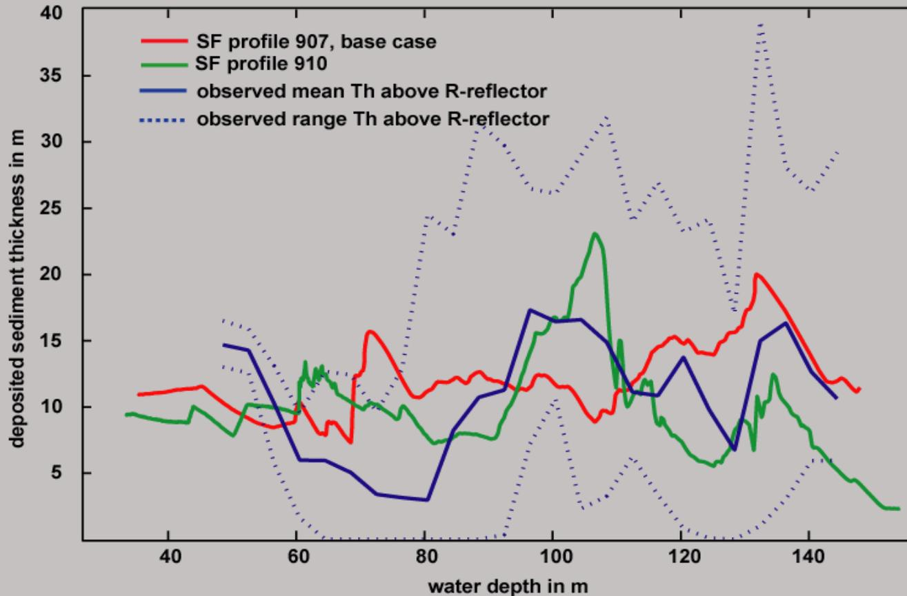
Red and green lines show the deposited sediment thickness over the entire SedFlux simulation against water depth. The 3D interpreted surface of the R-reflector depth is collapsed into a mean thickness of sediments above the R-reflector per water depth (blue line). The predicted SedFlux thickness matches the observed thickness rather closely and falls for the greater part well within the observed range (dotted blue lines).
