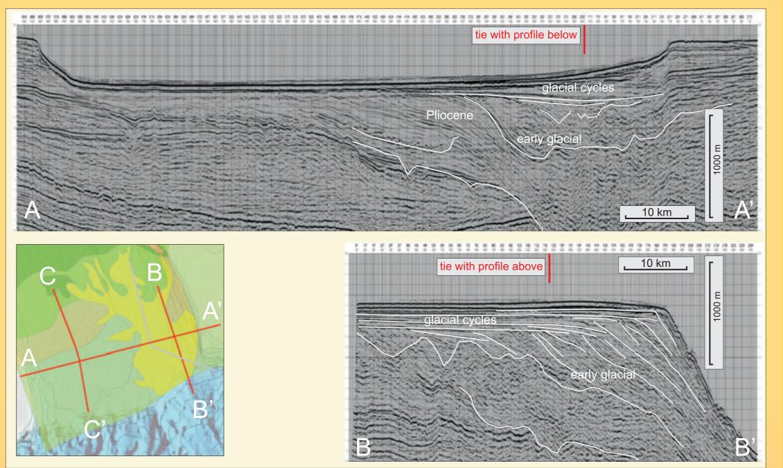
Figure 3. Multichannel seismic profiles help delineate various generations of cut in a large, previously unrecognized, canyon. Detailed Cenozoic mapping indicates a large Pliocene infill. Multiple tills bound by flat ice-stream cut beveling erosion surfaces help differentiate tills from sediments pre-dating glaciers reaching the paleo-shelf-break. The map (Fig. 2) traces the canyon at the level interpreted as base of glacial fill. The numerous glacial tills are mapped in detail (Fig. 12)
