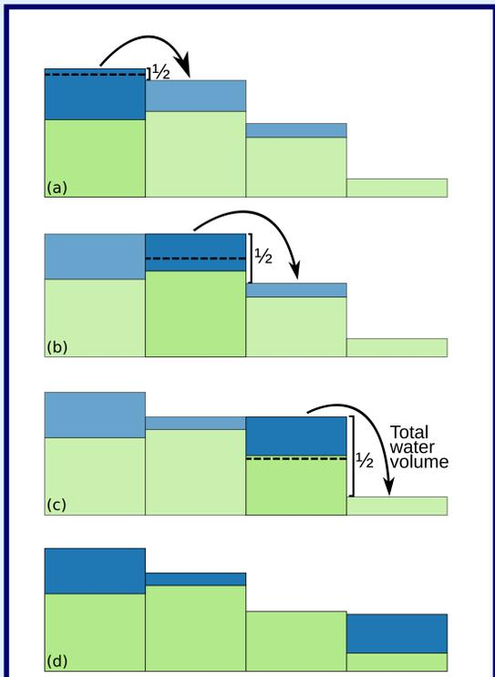
**Figure 2:** Water flow during a single iteration of FlowFill. Water moves starting with the highest cell and ending with the lowest. Each 'target cell' routes water into its steepest downslope neighbour. The amount of water moved is the min(all the water available, half the difference in elevation between the two cells). This latter criterion ensures numerical stability, but slows convergence towards a solution.
