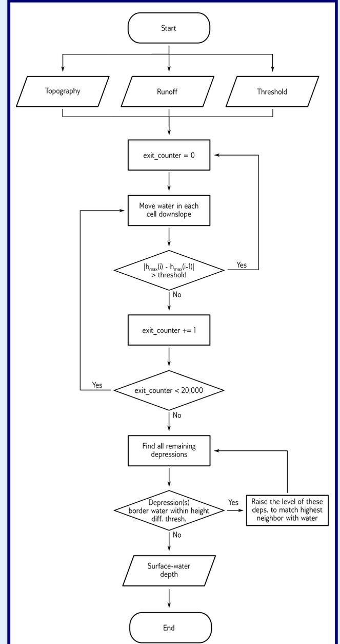
**Figure 5:** FlowFill flowchart. ' $h_{max}$ ' is the maximum amount of water moved from a single cell to another during each iteration ('i'). The majority of the runtime is spent sorting the cells into a queue and moving water from the highest cell to those below.
