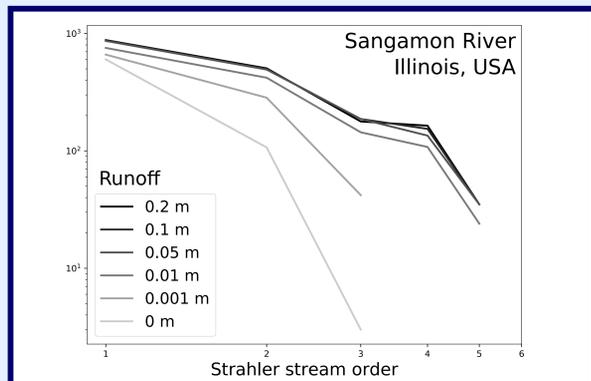
**Figure 4:** As more water is added to the landscape, more depressions are flooded and drainage integration (and therefore hydrologic connectivity) increases. More stream segments overall exist on the landscape, and they become more connected, increasing the fraction of higher-order streams.
