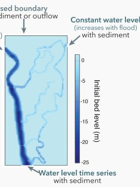
Sample model set-up for the Polder 32 case study. Water level time series contains either ebb-flood (tidal sites) or constant flood (fluvial) conditions.
