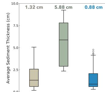
Median values of sedimentation along the cross-sections range from **0.88-5.88** cm/yr, higher rates of sedimentation due to greater SSC and more confined flow
