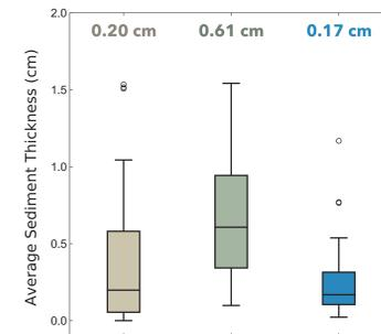
Median values of sedimentation along the cross-sections range from **0.20-0.61** cm/yr, lowest rates in all three model runs coincide with lowest SSC.
