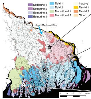
Output of cluster analysis of islands and channels in the GBMD. 5 primary zones are illustrated (estuarine, tidal, transitional, inactive and active fluvial).
