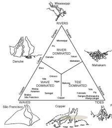
The GBMD is considered tidally-dominated, but it also receives a large amount of fluvially-driven discharge and sediment. Example Galloway diagram taken from Witek and Czechowski (2015).
