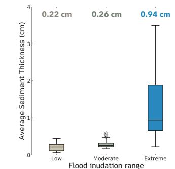
Median values of sedimentation along the cross-sections range from **0.22-0.94** cm/yr, similar to the fluvial case. Deposition is likely low due to high velocities and unconfined flow.
