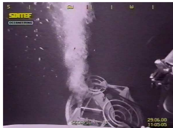
Fig. 4 Picture taken from the ROV of the discharge platform showing the gas bubble plume from the LNG experiment.
