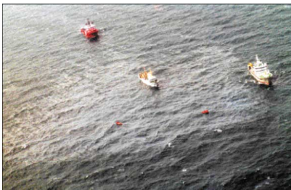
Fig. 3 Aerial image of surface slick from diesel discharge. Picture taken from the Norwegian surveillance aircraft June 27. The vessels seen on the picture are (from left to right): Far Grip , Håkon Mosby and Johan Hjort . The two small boats are sampling boats. The ROV on the Håkon Mosby was used to monitor the discharge.
