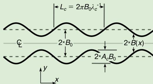
Figure 1. General planform geometry of variable width channels
