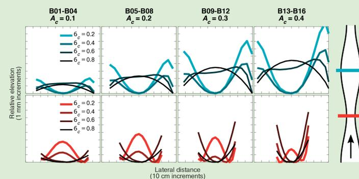
Figure 6. Cross-section profiles of the widest/narrowest channel sections from the B-Series final states. Vertical exaggeration of 100.
