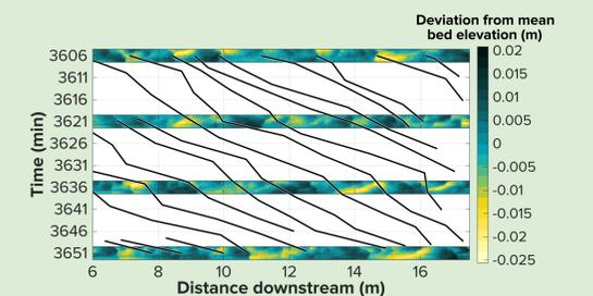
Figure 9. Gravel bedform migration in a straight-walled flume
