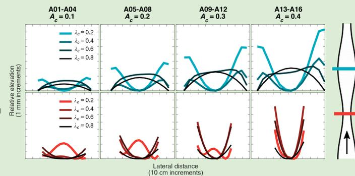
Figure 5. Cross-section profiles of the widest/narrowest channel sections from the A-Series final states. Vertical exaggeration of 100.
