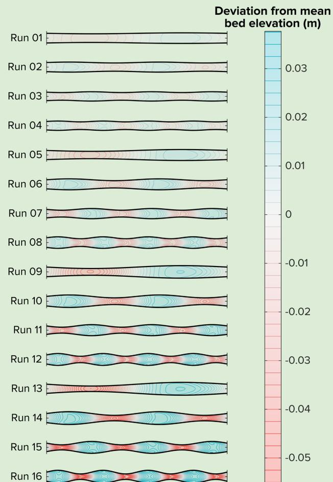
Figure 4. Detrended elevation maps for A-series. Vertical exaggeration of 10. Contour intervals of 2.5 mm.
