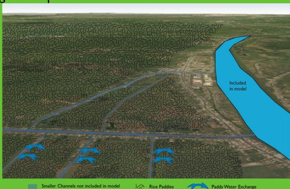
Figure 1: Included and excluded channel in current LISFLOOD-FP model and delineation of paddies
