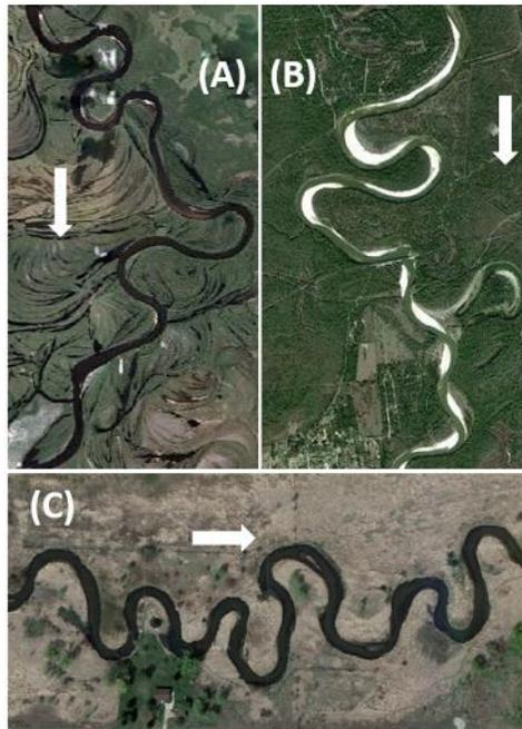
Figure 3.1. Meandering river reaches showing width variation. (a) Ob River, Russia. (b) Trinity River, Texas, USA. (c) Vermillion River, Minnesota, USA. Arrows indicate direction of flow. For scale, typical river widths are 150 m, 190 m, and 15 m for cases a), b) and c) respectively.
