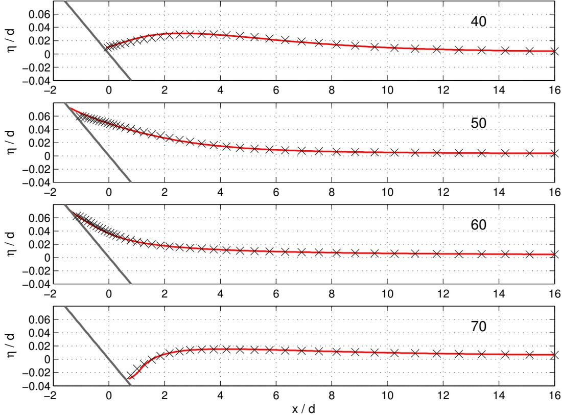
Figure 1: Water surface profiles for an initial solitary wave  $0.0185d$  high climbing up a 1:19.85 beach at  $t(g/d)^{1/2} = 40, 50, 60, 70$  (shown in a plot), black x - Cliffs numerical solution, red line - analytical solution. Plotted with Matlab script *plotprofiles0185-cliffs-vs-analyt.m*
