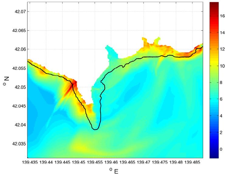
Figure 3: Maximal wave height in Aonae grid; colorbar - meters, black line - original shoreline before subsidence. Plotted with Matlab script *aonae\_inundation.m*
