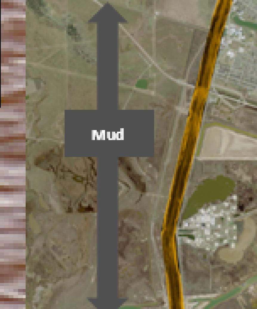
Figure 12: Side scan survey mosaic of the Brazos River from June 28, 2010 showing changes in dominant bottom sediment type. Mud area indicates the extent at which the null point migrates as the salt wedge moves with changes in
