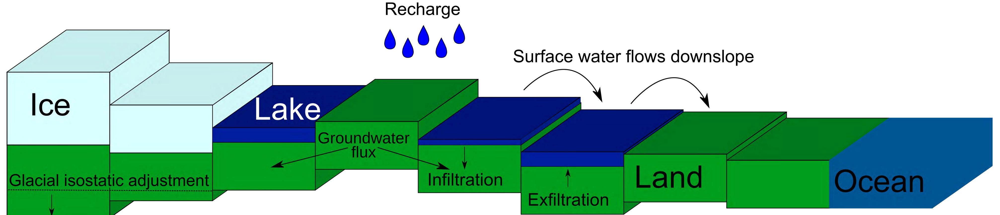
Figure 1: Model schematic showing both the groundwater and topography, adjusted according to glacial isostatic adjustment and changing sea level. Groundwater moves down hydraulic gradient and exfiltrates when it enters a cell that is not fully saturated in the groundwater. Lakes form in local basins, and additional water runs off to the ocean. Groundwater levels fluctuate with changing recharge and topography through time.
