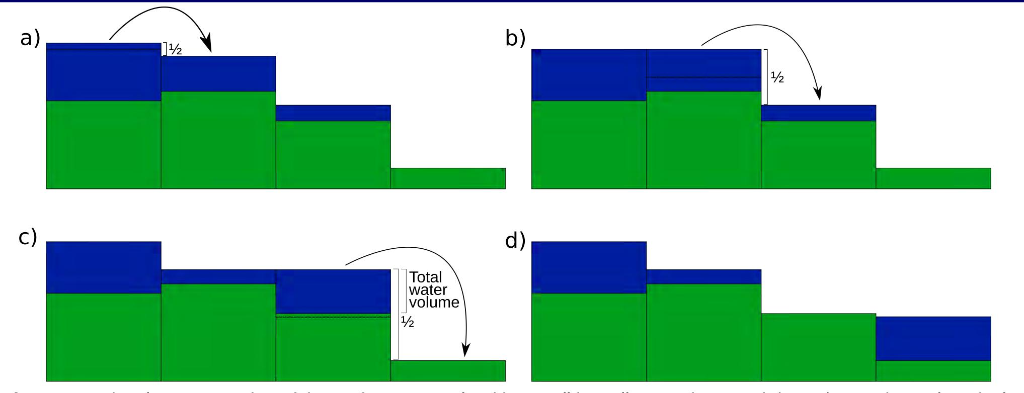
Figure 2: A visual representation of the surface water algorithm. Cell by cell, water is moved downslope, where slope includes both land and water. The steepest direction is selected, and then max(half the difference between the two cells, all the water in the cell) is moved to the downslope cell. From a to d, one iteration through the surface water array is shown. In the next iteration,
