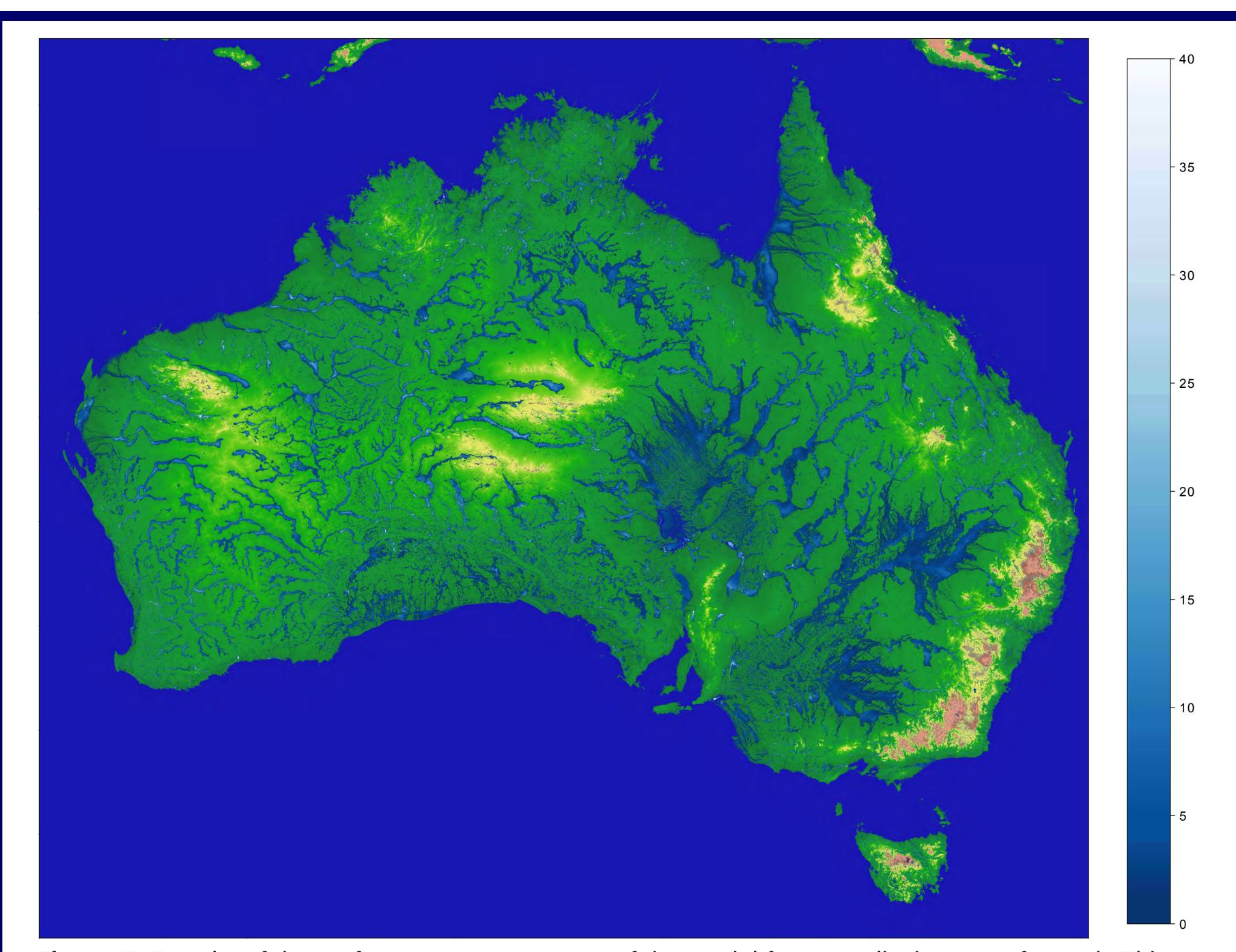
Figure 5: Results of the surface water component of the model for Australia (metres of water). This model can be run on a continental or global scale. While the results of the surface water component alone may be unrealistic - in this case, a combination of an overly large water input and a lack of infiltration and evaporation has resulted in an overestimate of Australian surface water - it does provide an interesting look at Australia's enclosed basins.
