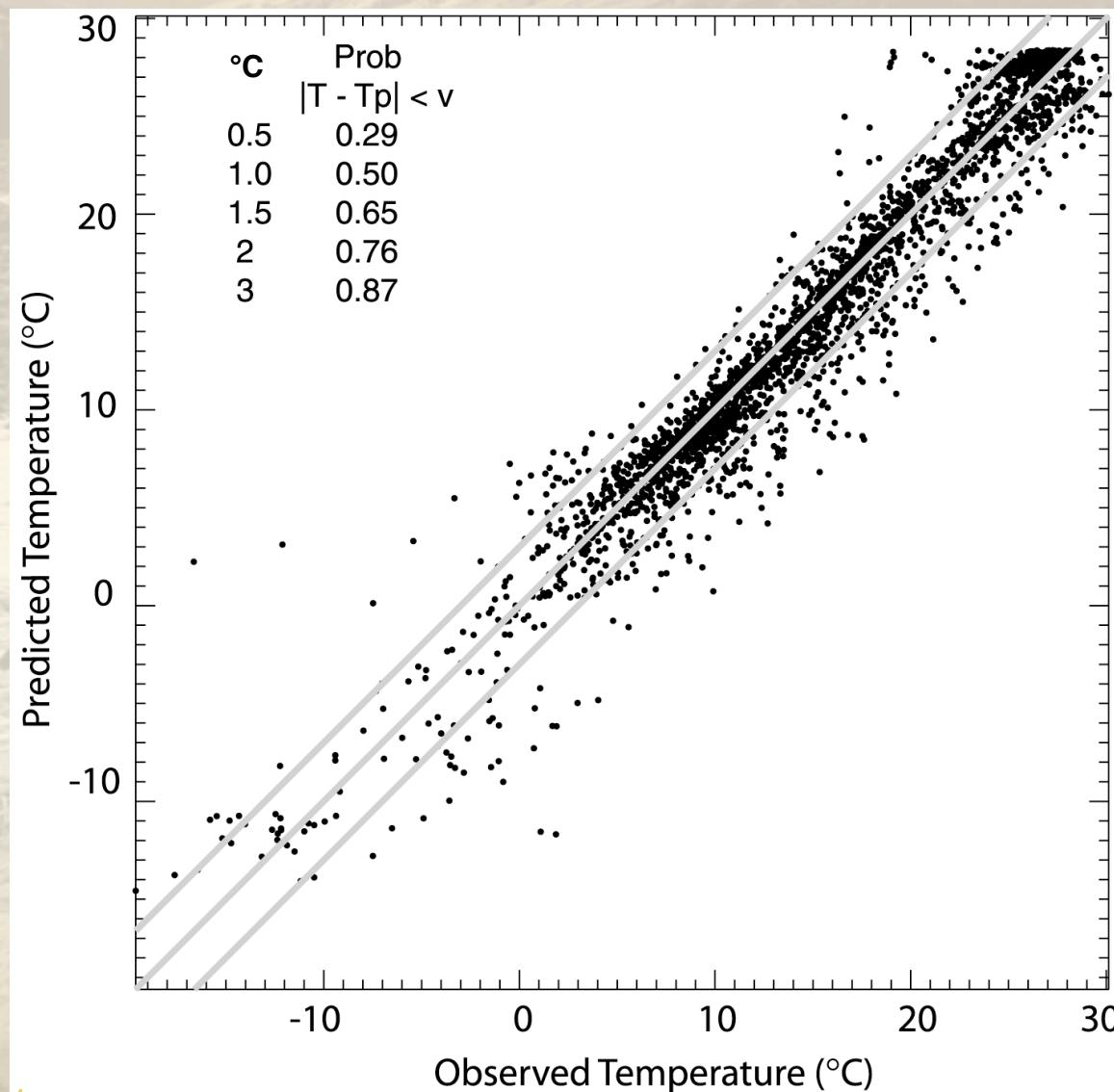
Observed versus predicted station temperatures. Half of the data falls within 1°C of prediction, and 82% falls within 2.5°C. Basin averaging of station temperatures reduces local variability and provides for basin-averaged values of  $\pm 1.5^{\circ}\text{C}$ .
