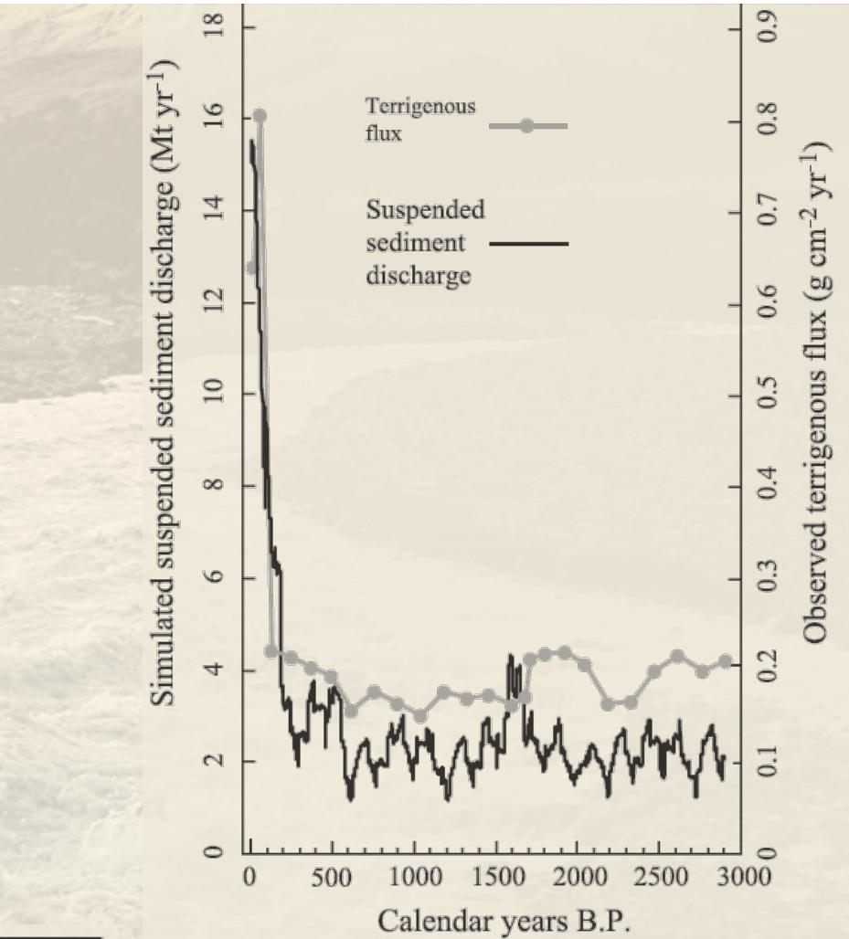
**Figure 10.** Comparison of the late Holocene suspended sediment discharge (99-yr running mean) from the Waipaoa River system computed using HydroTrend and the observed rate of terrigenous mass accumulation on the middle shelf at core site MD972122 [after Gomez *et al.*, 2007] (see Figure 1 for location).
