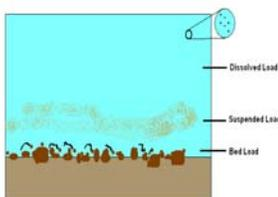
Fig 1: Different sediment movement in rivers (Ritter, 2006)
