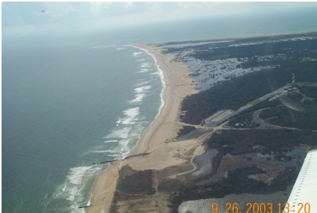
Cape Hatteras, NC, after Hurricane Sandy made landfall nearby in 2003, showing storm-related flooding, old groynes that have influenced coastline morphology, and a landmark lighthouse that had recently been transported a kilometer farther inland after a century and a half of chronic shoreline erosion threatened it.
