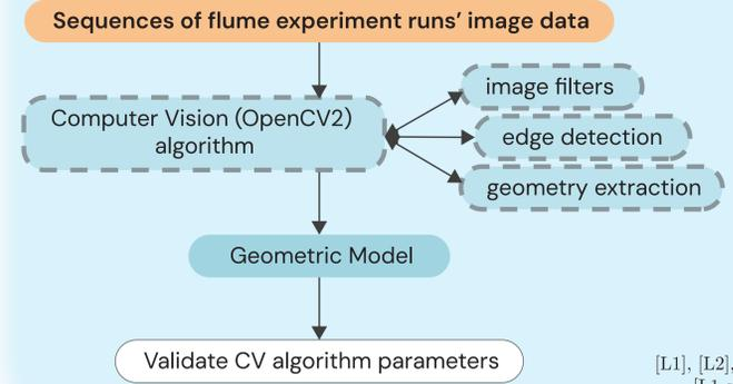
Figure 4: Detail flowchart of the Geometric Model
