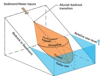
Figure 1: 3D geometry diagram representation of the Enthalpy process-based model
