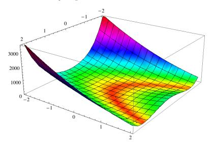
Figure 1. The Rosenbrock function, a classic test problem in optimization.
