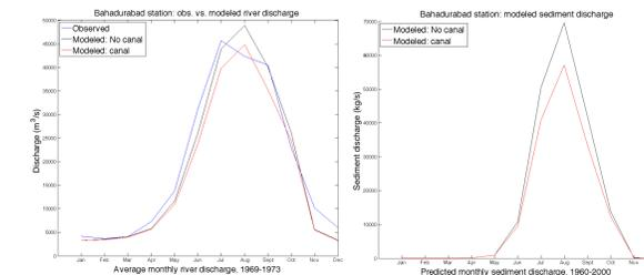
Fig. 9 a) Observed vs. modeled river discharge for Bahadurabad station with and without link #13. b) Predicted sediment discharge change due to link #13.
