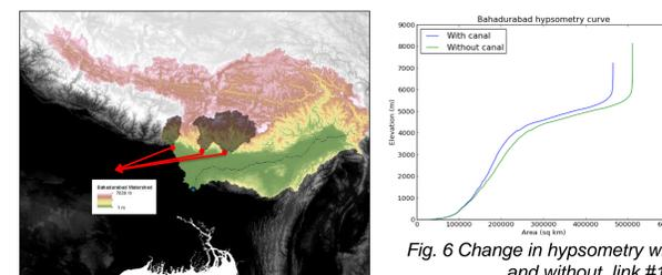
Fig. 5 Watershed of the Brahmaputra River above Bahadurabad gauging station. Shading shows areas effectively removed from the watershed by proposed canal #13, the Manas-Sankosh-Tista-Ganga link, which would transport water from the shaded areas out of the Brahmaputra watershed and into the Ganges river and further south.
