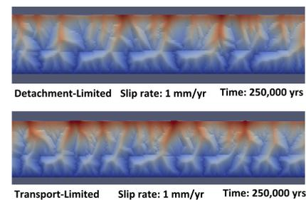
Figure 7. In the detachment-limited case, rivers flowing along the fault are able to sustain longer offsets than rivers in the transport-limited case are.
