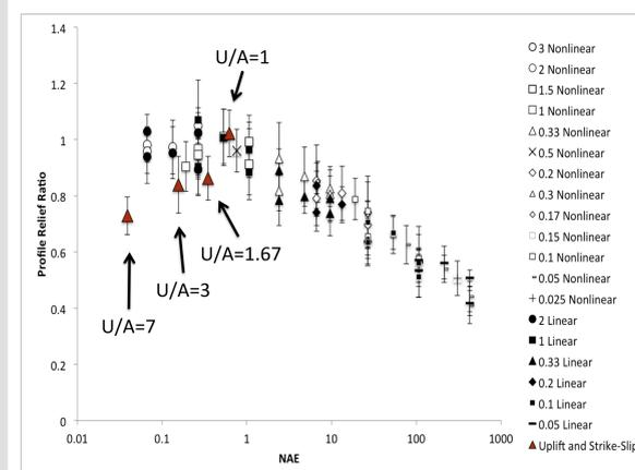
Figure 4. Plotting  $N_{AE}$  versus PRR shows the inverse relationship between  $N_{AE}$  and PRR. In our model setup, PRR reaches a maximum around or slightly above 1. The symbols in red are out new, differential-uplift runs.
