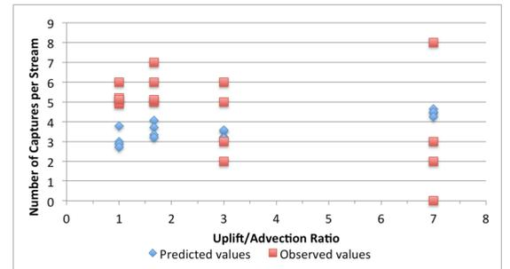
Figure 5. The number of stream captures occurring on certain streams in the model runs, during the time it takes each run's fault to slip 500m. These values are compared to predicted values, which are simply the number of times streams are expected to be juxtaposed, based on the drainage spacing of the model.
