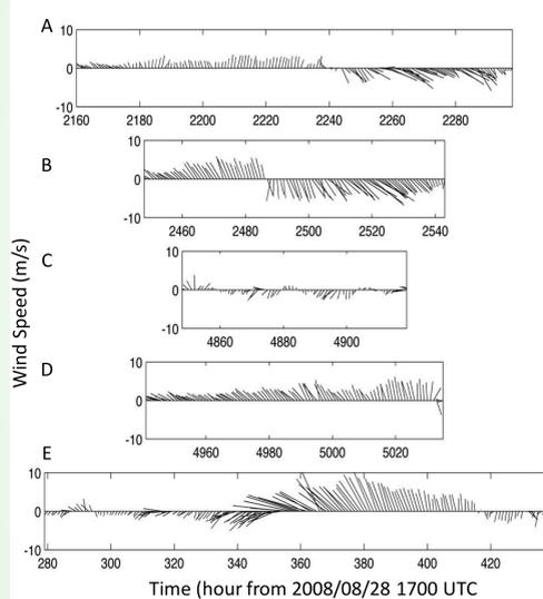
Fig. 2. Wind structures: A) typical cold; B) strong cold front; C) minor cold front with offshore winds; D) cold front with onshore winds; E) Hurricane Ike.
