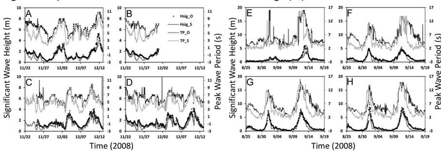
Fig. 4. Comparison of modeled and simulated significant wave height (m) and wave periods (s) at NOAA buoys stations.
