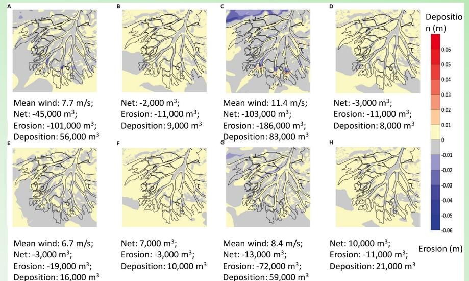
Fig. 5. Morphological changes and sediment balance during A) cold front CF 9 including winds and waves; B) CF 9 excluding winds and waves; C) CF 11 including winds and waves; D) CF 11 excluding winds and waves; E) CF 20 including winds and waves; F) CF 20 excluding winds and waves; G) CF 21 including winds and waves; H) CF 21 excluding winds and waves.
