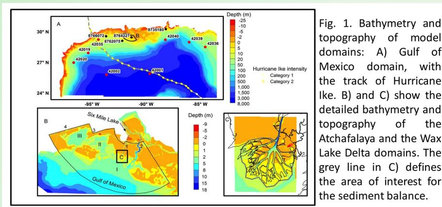
Fig. 1. Bathymetry and topography of model domains: A) Gulf of Mexico domain, with the track of Hurricane Ike. B) and C) show the detailed bathymetry and topography of the Atchafalaya and the Wax Lake Delta domains. The grey line in C) defines the area of interest for the sediment balance.
