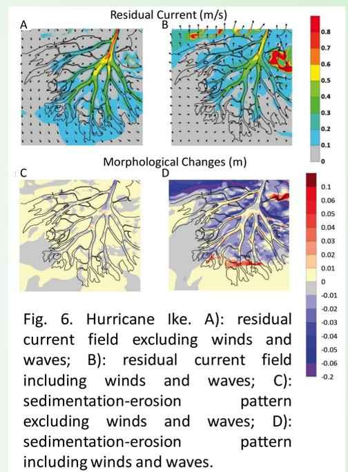
Fig. 6. Hurricane Ike. A): residual current field excluding winds and waves; B): residual current field including winds and waves; C): sedimentation-erosion pattern excluding winds and waves; D): sedimentation-erosion pattern including winds and waves.
