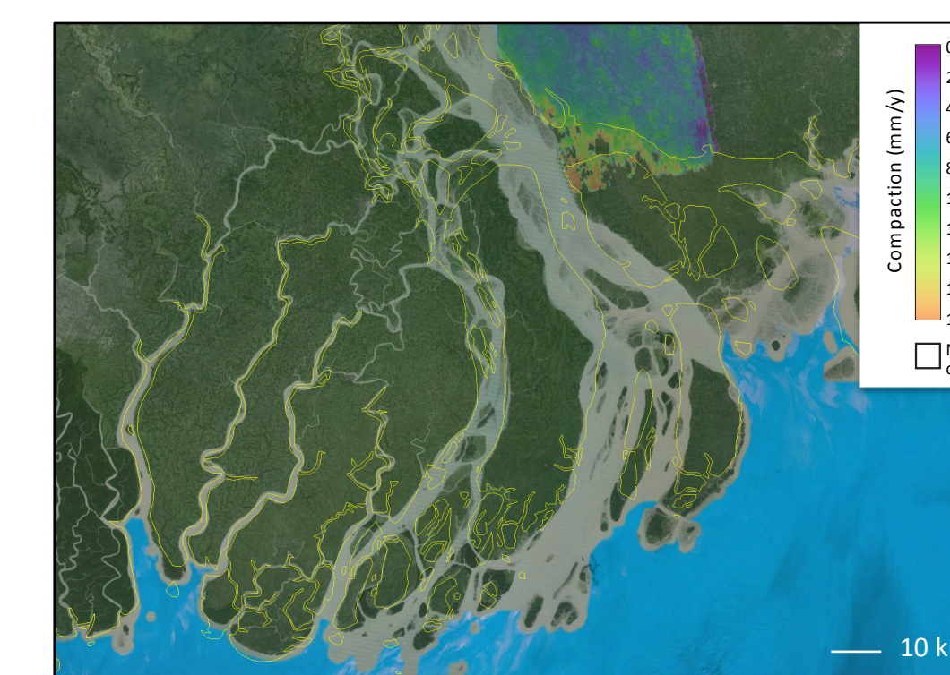
Fig 10. The coastline from 1944 shows a branch of the Meghna that filled with sediment during the 1950 Assam Earthquake. This newly deposited sediment is rapidly compacting; InSAR captured the boundary.
