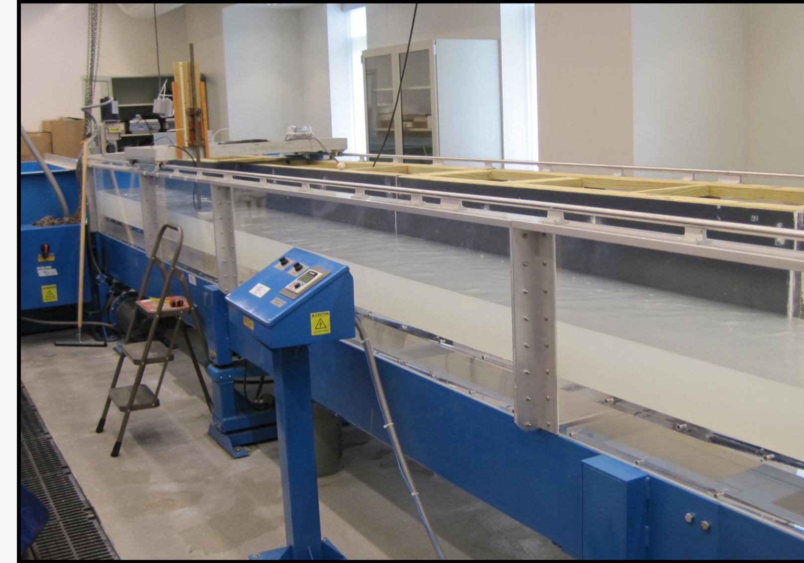
Fig. 4- Recirculating flume, 8 m x 1 m x 0.4 m
