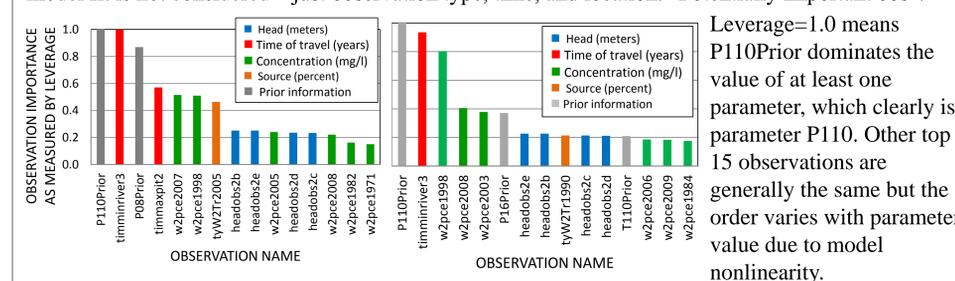
Timminriver3, the time it takes the fastest particle to travel from the river to well 3, is most important.
