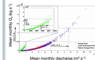
**Figure 5b.** Sediment rating curves for each of the three sub-systems based on 100-year HydroTrend simulations. Each monthly sediment load is plotted versus the monthly water discharge, illustrating the enormous spread in events for these monsoon-driven rivers
