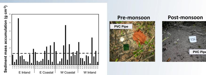
**Figure 3.** 2008 tidal delta direct sedimentation measurement results: 100% trap recovery; all sites received new sedimentation; overall mass accumulation average:  $1.3 \pm 1.1$  g cm<sup>-2</sup> (dashed line); <sup>7</sup>Be results: 63% sourced from monsoon floodpulse; riverine sediment reworked onto tidal plain by 2-4 m tidal range + set up; **regional vertical accretion:  $1.1 \pm 0.9$  cm y<sup>-1</sup>**
