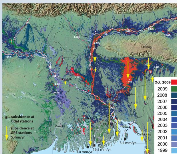
**Figure 1.** Flood maps constructed from MODIS satellite imagery show ~52,800 km<sup>2</sup> of flooded lands in the delta (>100 m a.s.l.) between 2000-2009 (flood area data from Flood Observatory, hosted at the CSDMS: <http://floodobservatory.colorado.edu/>). GPS-based short-term subsidence. Sediment delivery to the G-B delta's surface occurs through overbank flooding of the rivers and tidal reworking.
