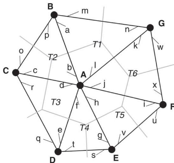
Sample mesh consisting of 7 nodes (A-G), 6 triangles (T1-T6), and 24 directed edges (a-x) (from Tucker et al., 2001).
