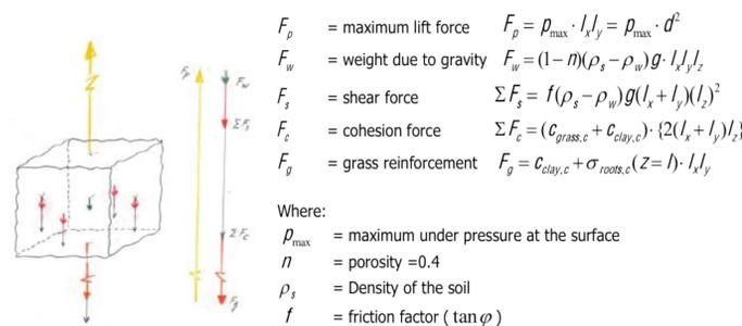
Figure 3. Forces on a soil cube (Hoffmans, et al., 2009)
